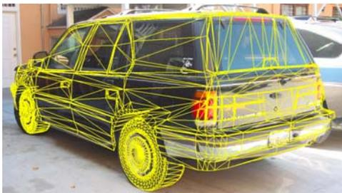
Figure 4. Projected 3D model after modeling
