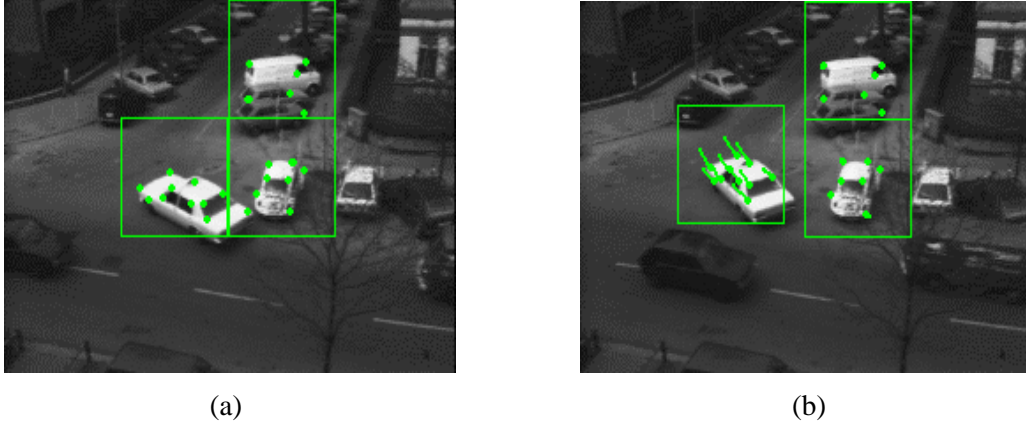
Figure 2. Hamburg Taxi Sequence: (a) first frame with detected region and point features, and (b) motion results at 20 th frame.
