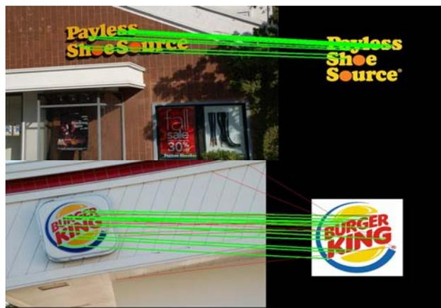
Figure 10(c): Real and computer-generated images test result. Right side training images are computer-generated images downloaded from the Internet. In the “Burger King” example, red (dark dash) lines are outliers removed by consistent check.
