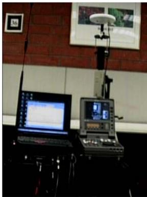
Figure 8. Image capturing system. The major components are a video recorder and an omni-directional camera. A differential GPS shown in the Figure is not used for pose estimations but used for measuring ground truths.
