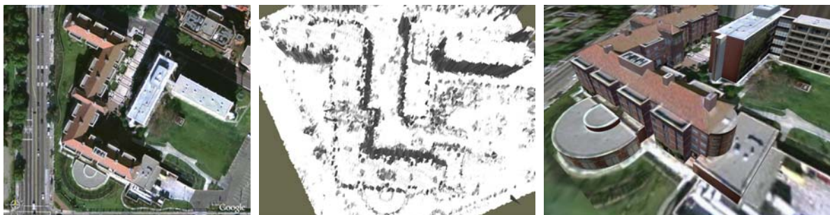
Figure 1. From left to right. (a) an input aerial image; (b) input LiDAR data; (c) the hybrid modeling result.
