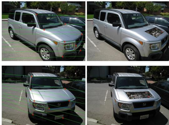
Figure 1: Epipolar lines (left) and augmented annotations (right) for stereo images with large viewpoint change.
