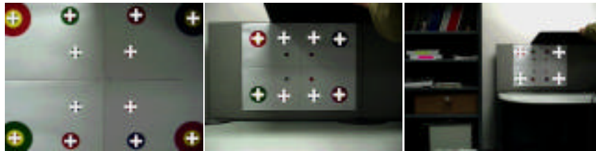
(a) Distance 3 feet - All three level fiducials are detected (b) Distance 6 feet - The second and third level fiducials are detected (c) Distance 12 feet - Only the third level fiducials are detected
