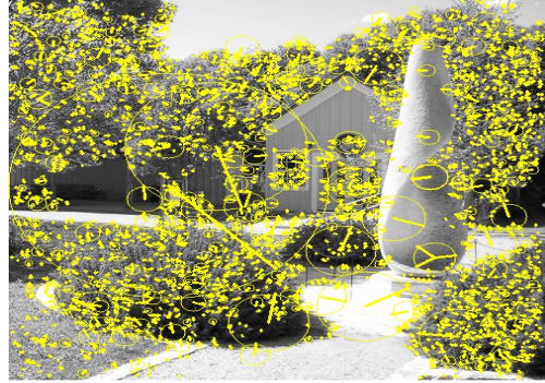
Fig 2: Detected salient features with feature locations, dominant orientations, and scales
