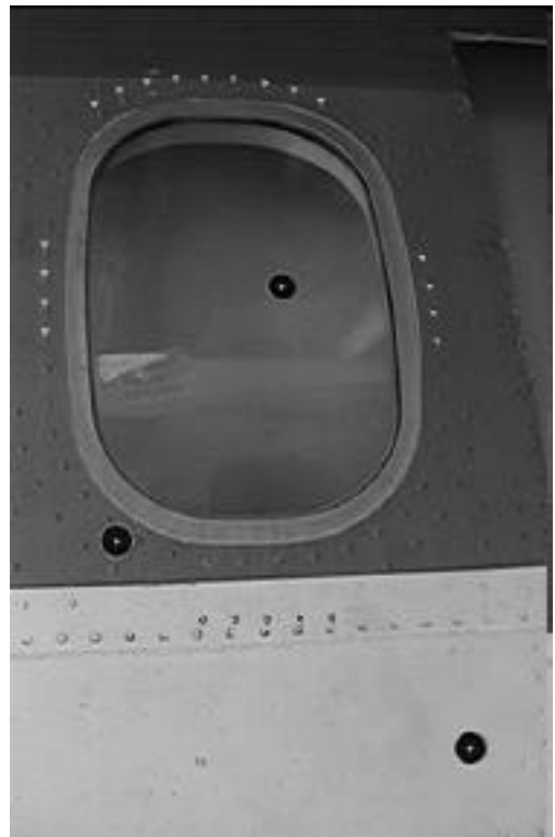
Fig. 6 - Three fiducials and annotation around window frame from two vantage points
