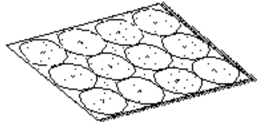
Fig. 4 - Elliptical kernel extents for one pass showing independence of every fourth voxel in x and y
