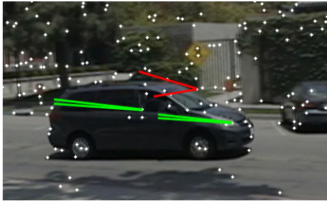
Figure 2. Bidirectional Optical Flow. For three detected keypoints we show the optical flow vector in both directions. For two of those keypoints (green vectors), the vectors match and are deemed valid. For a third, however, they do not match (red vectors) and the point is discarded.
