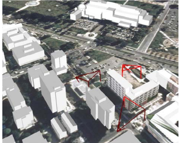
Figure 2 - An AVE system screen snapshot showing three video projections within a campus area.
