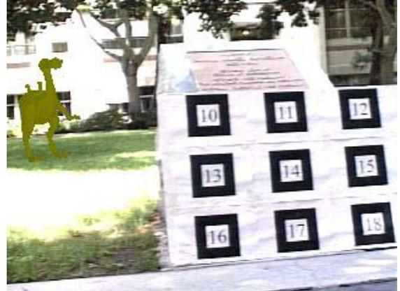
Fig. 6 (a) 200<sup>th</sup> frame, camera pose was estimated from pre-calibrated landmarks on the board.
