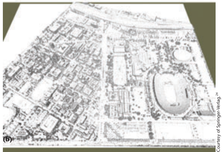
7 A Lidar capture system: (a) an aircraft carrying the system flies over an area, emitting pulses and measuring their reflection. (b) A Lidar-generated digital elevation model of the USC campus and surrounding area.
