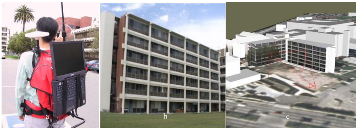
Figure 9 - Texture painting with real data. (a): Portable video acquisition and tracking system. (b): One frame of the captured video. (c): Rendered scene of USC campus with live video painting.
