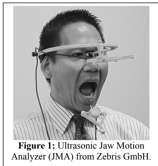
least three points relative to this plane during jaw motions are saved in an ASCII file. The three points are the two condylar points and the base center of the T-attachment pointer attached to the jig.
