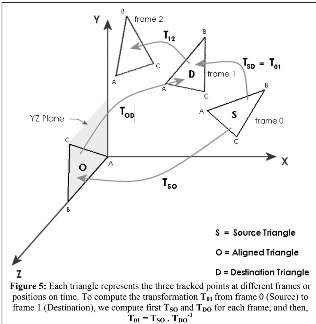
The transformation matrices  $T_{01}, T_{12}, \dots, T_{(n-1)n}$  were recursively applied to the model of the mandible which is treated as a single object in 3D Studio Max.
