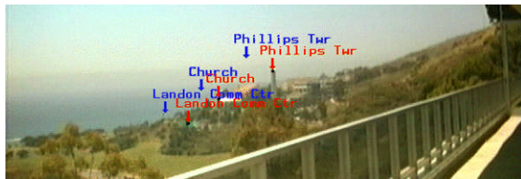
Figure 6: Virtual labels annotated over landmarks for video sequences showing vision-corrected (red labels), and inertial only (blue labels) tracking results.
