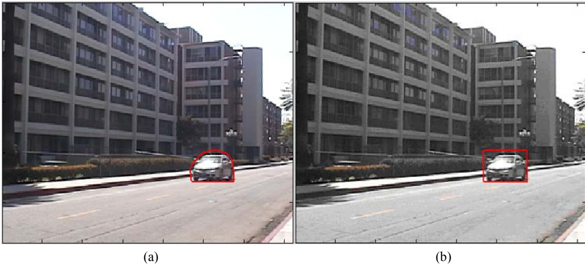
Figure 2: a moving vehicle is detected and modeled as a convex hull with 18 points (a), and a rectangular polygon (b)
