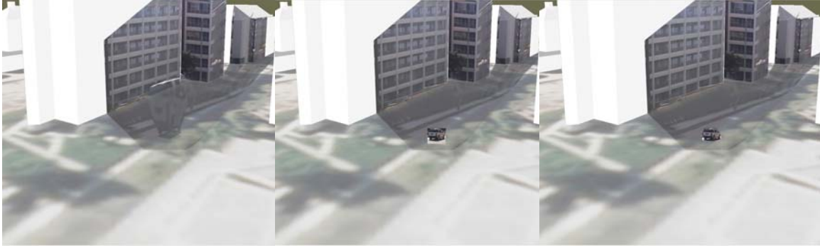
Figure 4: (a) An image projection of a moving car without a dynamic model results in a distorted presentation, (b) the moving car is modeled as a rectangular polygon, and (c) is modeled as a convex polygon.
