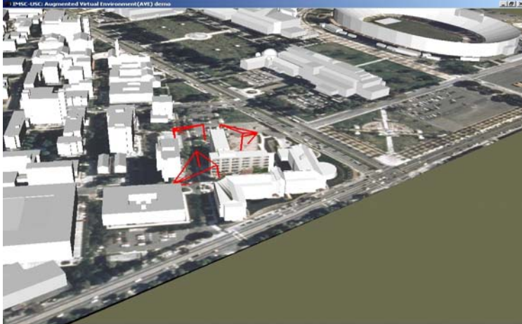
Figure 1: An AVE system showing projections of three video streams (wire-frame frustums) and an aerial photograph within the USC campus area.
