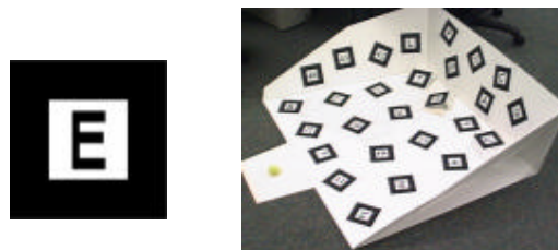
Figure 2. (a) Fiducial, (b) board with calibrated fiducials.
