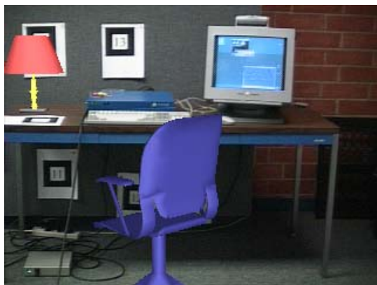
(c) The virtual chair and lamp from another viewpoint where none of pre-calibrated landmarks are observed. Camera pose is computed only from autocalibrated features.
