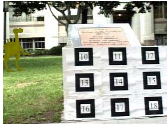
(a) Camera pose was estimated from pre-calibrated landmarks on the board.
