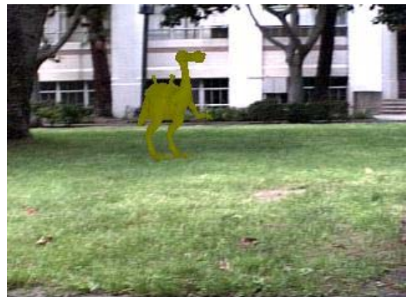
(c) Camera pose was estimated from auto-calibrated line features. None of the pre-calibrated landmarks were observable.
